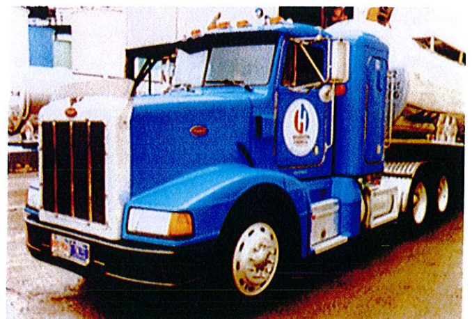
The chemical shipper has two Peterbilt conventional tractors with Cummins L10 330-hp engines, Fuller 10-speed transmissions, and Eaton 40,000-lb tandem-drive axles.
