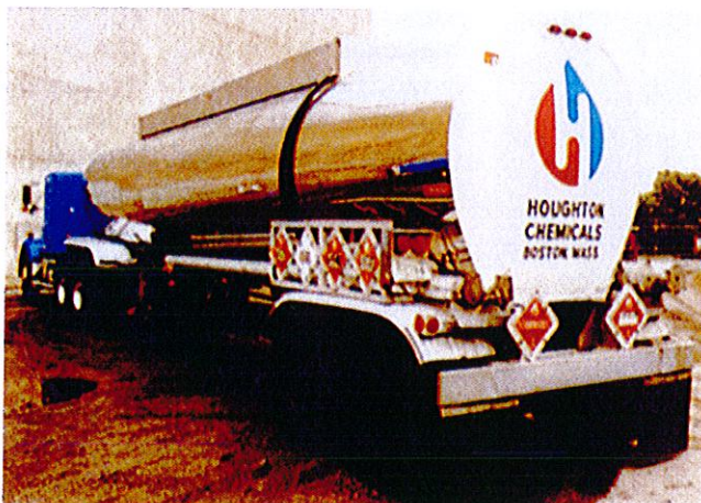
Most Houghton Chemical transports are multicompartiment Fruehauf MC307 double conical tank trailers with capacities up to 8,300 gallons. The trailers are equipped with intransit heat.
