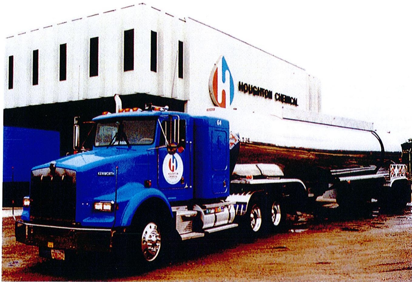
Houghton Chemical has seven bright blue Kenworth T800 tractors dressed up with polished aluminum wheels that make a positive, striking impression when pulling into a customer's yard to make a delivery. The tractors have Cummins engines, Fuller 10-speed transmissions, and Eaton 40,000-lb tandem-drive axles.
